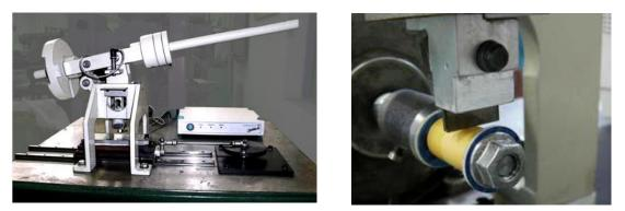
Figure 3. The basic equipment (Zsidai et al 2006; Lefánti et al 2011) and the clamped ceramic and steel specimens developed to the frictional test.
