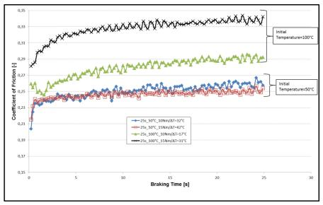
Figure 5. Curves of coefficient of friction for different initial temperature and torque.
