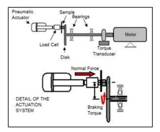
Figura 2. Scheme of the laboratory-scale tribometer.
