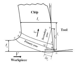
Figure 3. Parallel-sided shear zone model of Oxley [13].
