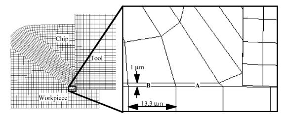
Figure 5. Link elements in the finite element model [8]
