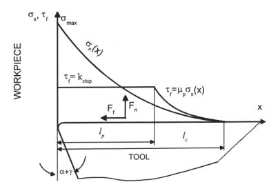
Figure 2. Normal and frictional stress distribution at the tool rake face [12].
