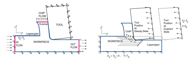
Figure 1. Finite element model for ALE formulation with: a) Eulerian and Lagrangian boundary conditions (with predefined chip) [11, 14], and b) pure Lagrangian boundary conditions [14].
