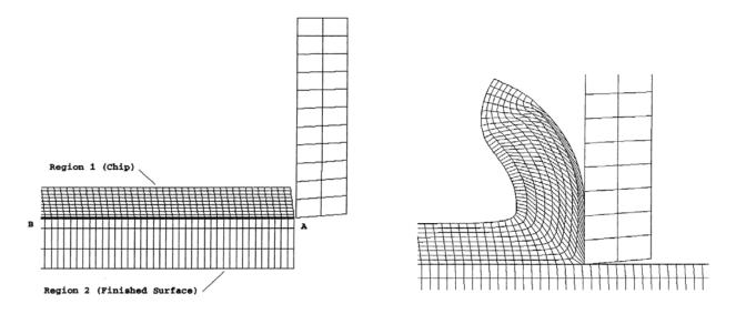
Figure 4. Left: Undeformed mesh with indication of node separation line (AB). Right: deformed mesh at steady-state cutting [7]
