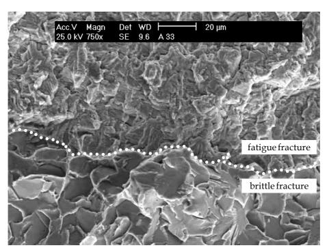
Figure 11: SEM micrograph of the boundary between the fatigue crack and the forced brittle fracture (magnification 750x).
