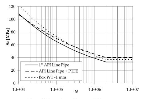
Figure 12: Comparison of the mean S-N curves.
