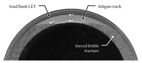
Figure 6: Fracture surface of a 1" API Line Pipe specimen with PTFE.
