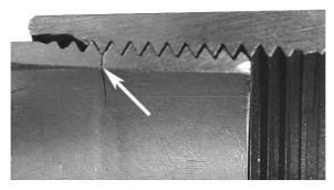
Figure 3: Fatigue crack initiated at the LET of the pin of a standard 1" API Line Pipe specimen.
