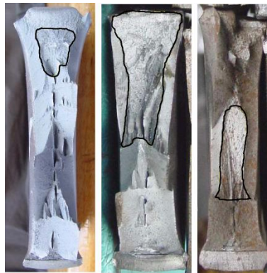
Figure 4. Three types of abnormal fracture appearance in DWTT specimens [6].
