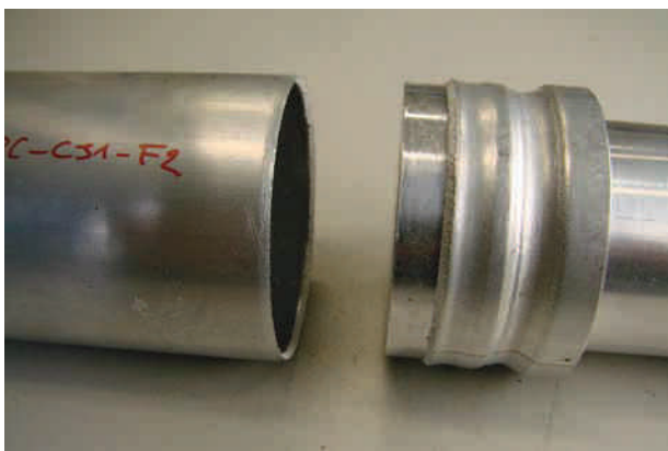
Figure 10: Specimen after tensile test: joint failure occurs due to shearing at the upper edge of the first groove
