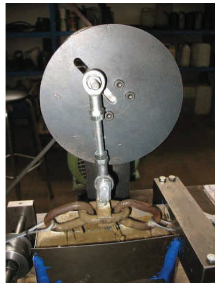
Figure 8: open chain cycle test rig developed at Laboratory Soete [8]
