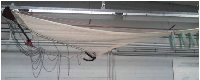
Figure 2: small model of a beam equipped with tickler chains [1]
