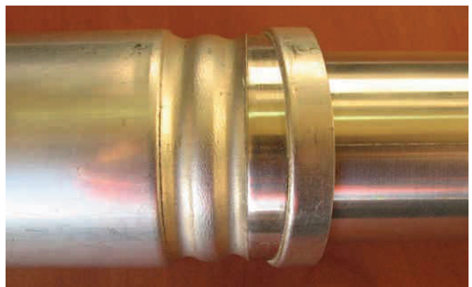
Figure 11: Mandrel with sharp edges cuts the tube
