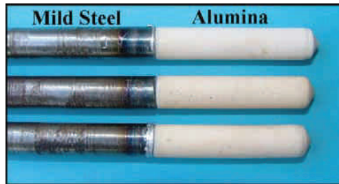
Fig. 3: Successful friction welds of alumina to mild steel (5)
