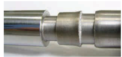
Figure 15: Shearing of tube metal during tensile test
