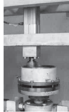
Figure 6: metal pin pressed against different kinds of gravel [3]
