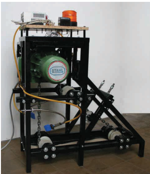
Figure 7: closed chain cycle test rig developed at Laboratory Soete [7]
