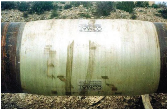
Figure 17: Demopipe composite crack arrestor before and after full-scale burst test [16]
