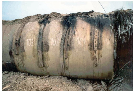
Figure 17: Demopipe composite crack arrestor before and after full-scale burst test [16]
