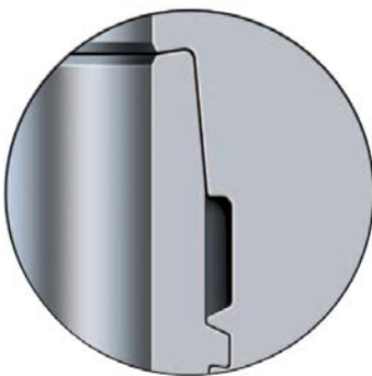
Figure 16: A lubricant relief groove avoids pressure buildup caused by grease. (Seal lock Apex, Hunting)
