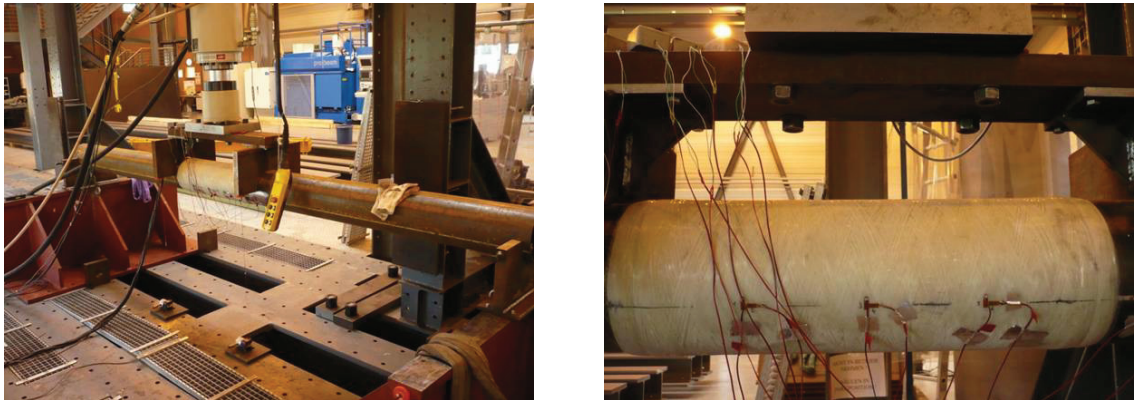
Figure 7: Four point bending setup (left) and strain gauge arrangement (right)
