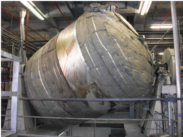
Figure 1: One of the four tumble dryers (capacity of 44m 3 ) at the Spinning Division of Sioen Fibres.
