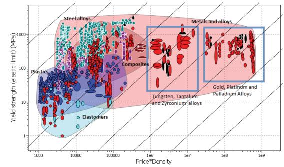
Fig. 3 Materials Selection Chart: evaluation of strength and cost
