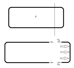
Fig. 2: Axial stress in the cylinder of a thin-walled pressure vessel.
