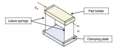
Figure 11: Fretting fixture based on a flexure mechanism [1]
