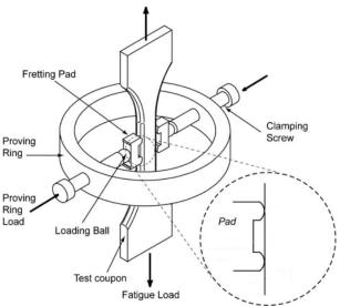
Figure 4: Proving ring test equipment
