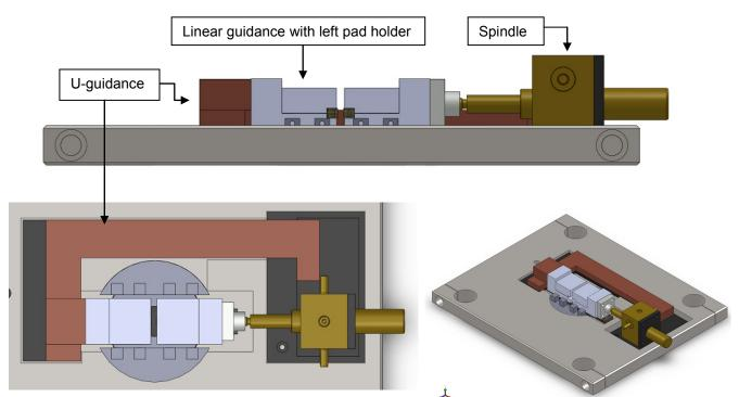
Figure 8: Concept 1: fretting fixture based on linear guides
