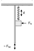
Figure 5: Impose of the relative displacement d through a spring system
