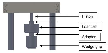
Figure 7: Specimen grip structure
