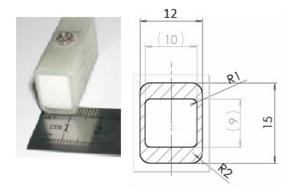
Figure 9: Artificial bone specimen and the dimensions [19].
