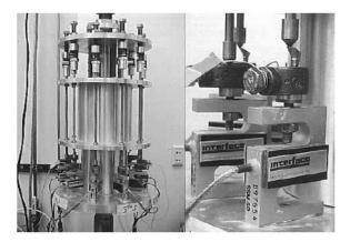
Figure 10: Carousel-type fatigue testing device [8]
