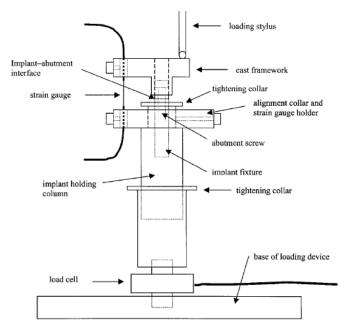
Figure 11: Solenoid driven dynamic loading test apparatus (schematic) [10]
