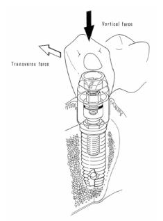
Figure 4: Vertical and transverse forces from occlusion acting on an implant prosthesis [7].
