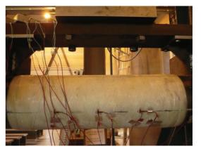
Figure 7: Four point bending setup (left) and strain gauge arrangement (right)
