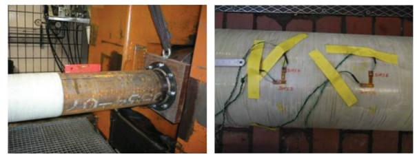
Figure 3: Clamping support (left) and strain gauge arrangement (right)
