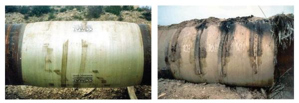
Figure 17: Demopipe composite crack arrestor before and after full-scale burst test [16]
