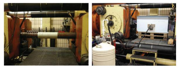
Figure 2: Tensile test setup for room temperature (left) and lower temperatures (right)
