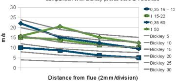
at higher pressures the velocity decreases more rapidly than the Bickley law, possibly due to the jet flow going fully turbulent.
