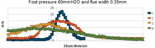
Jet transversal velocity profiles at various distances from the flue (2mm/division) Foot pressure 60mmH2O and flue width 0.35mm
