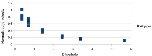
Normalised jet velocities at various wind supply pressures (mmH2O) against Dflue/toe
