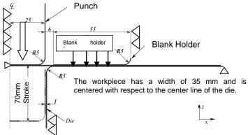
Figure 3. The NUMISHEET'93 benchmark geometry; (units: mm)
