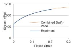
Figure 9. Combined Swift-Voce vs. experimental stress-strain curve.
