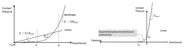
Figure 6. Linear and non-linear pressure-overclosure relation (left) and exponential (soft) contact pressure-overclosure relationship (right) [3]
