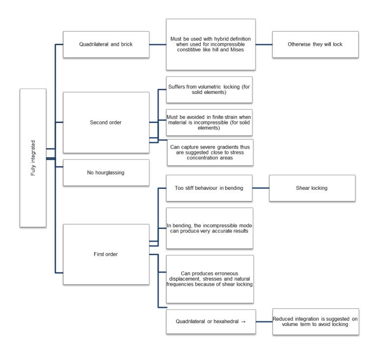
Figure 15. Guidelines for using fully integrated elements
