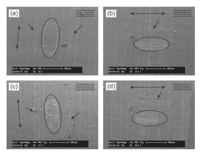
Figure 4. SEM images of the wear tracks of the carbon fibre reinforced epoxy after 40,000 cycles of reciprocated sliding against stainless steel with (a) anti-parallel and (b) parallel orientation, and alumina with (c) anti-parallel and (d) parallel orientation
