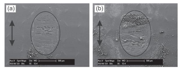
Figure 3. SEM images of the wear tracks of bulk epoxy against alumina after (a) 40,000 cycles and (b) 100,000 cycles
