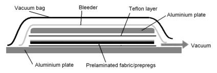
Figure 1. Carbon fibre reinforced epoxy's production set-up
