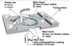
Figure 1. The position and dimension of specimens at pin-on-disk testing system.
