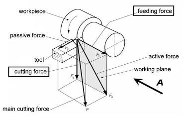
Figure 2. Cutting force components (ISO 3002/4, DIN 6584).
