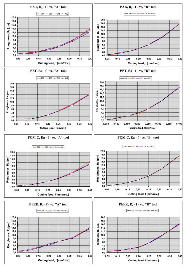
Figure 2. The results of R<sub>a</sub> in case of "A", "B" tools
