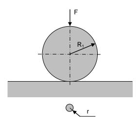
Figure 1. Contact area in a sphere-plane contact
