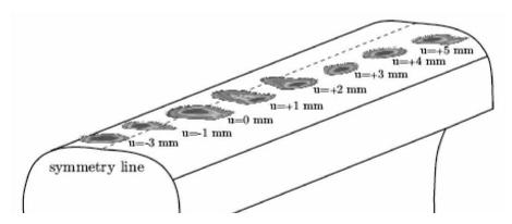
Figure 3. Comparison of the position and the shape of the contact area, depending on the variation of the lateral shift u (positive towards the gauge face) [9]
