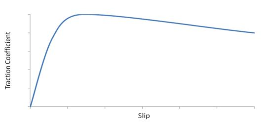
Figure 5: General curve of traction coefficient in function of slip
