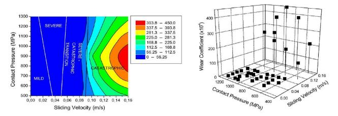
Figure 9: Wear coefficient maps for standard carbon steel. left: contour plot, right: 3D plot [17]
