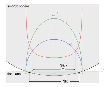
Figure 6: pressure (p) and shear (q) distribution in a static contact area
